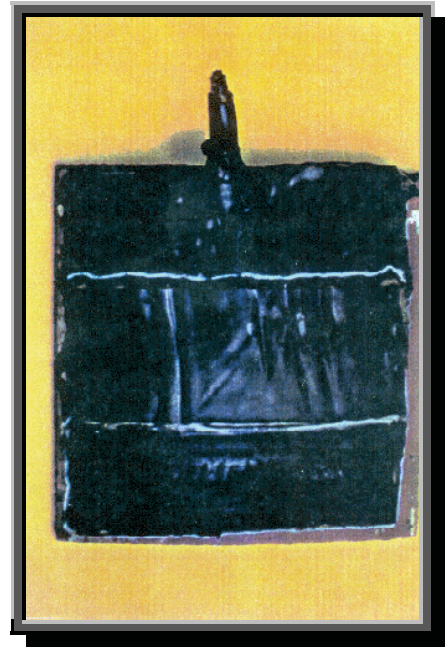
White ink marks remain in place proving that material maintains its original position after 28 days of destructive testing.
