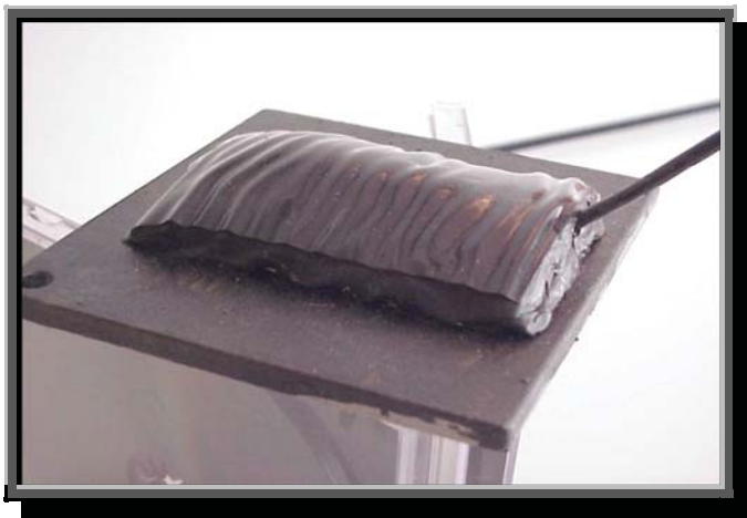
Figure 1-4. Thermite weld coated with the KEMA 250-12 Module Sealant system.
